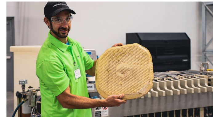
LiTDC technician showcasing a filter press cake; Thacker Pass is being designed as a zero-liquid discharge process to maximize water recycling and reuse
